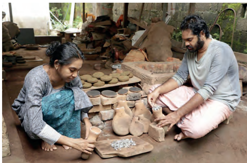
Above: The metallic disc created by the alloy that eventually becomes the mirror. Right: Artisans at work with the alloy prepared by mixing copper, tin and zinc in specific proportion
