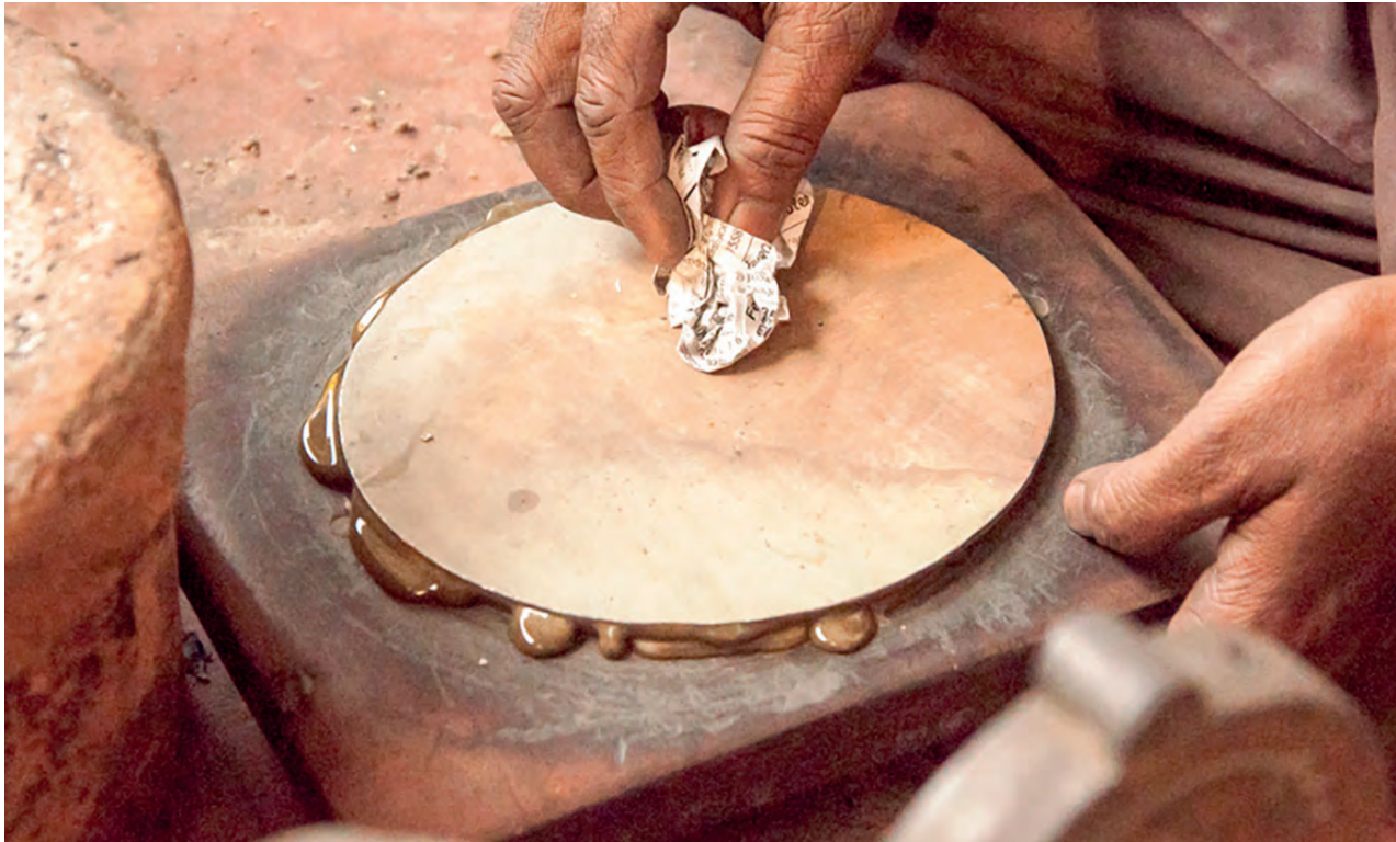
The polishing that creates the mirror from metal is a labour-intensive process comprising different stages
