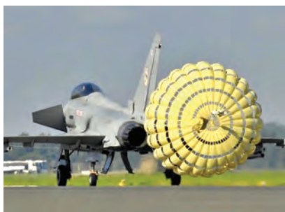
Hybrid Brake Parachute to assist the safe landing of Tejas has been indigenously developed
